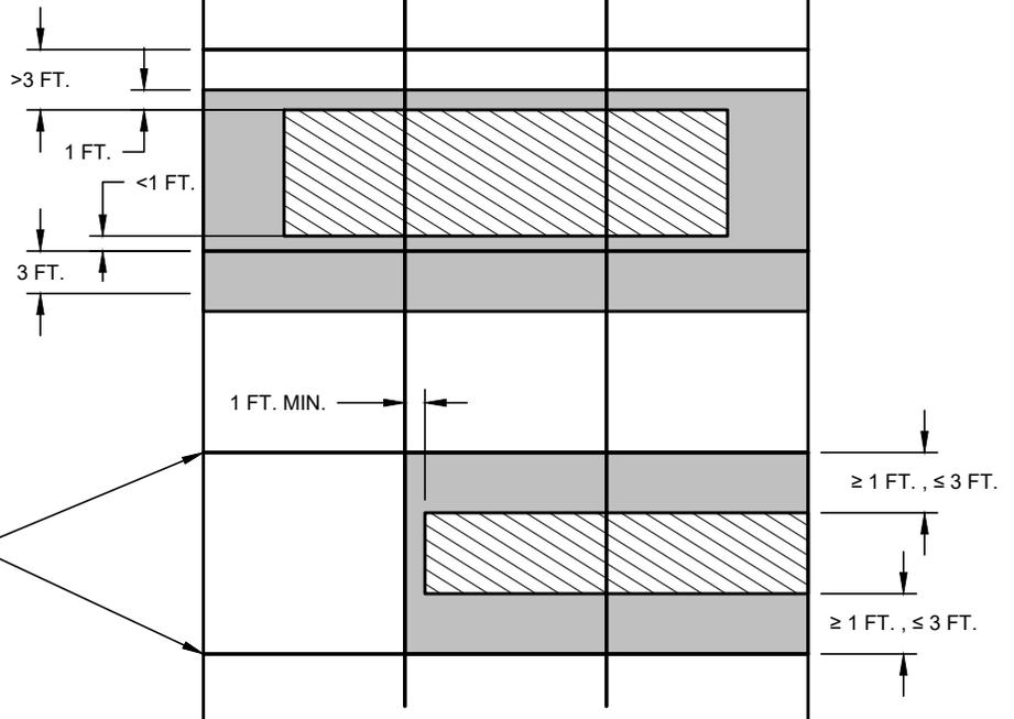
**CONCRETE ALLEY CUT REPAIR REQUIREMENTS**
