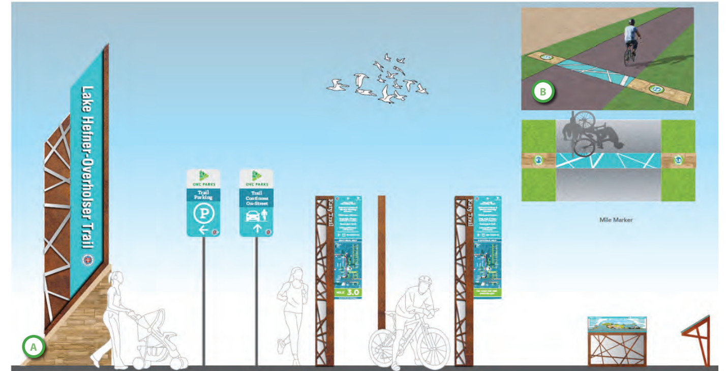
Trails system brand created as part of a wayfinding plan. Includes various gateway, directional, and interpretive signage, and corresponding trail markings within and adjacent to the trail surface. Branding elements are applied to each new trail segment according to placement plans that are incorporated into design and construction drawings. Elements from above (A) and (B), being installed below.
