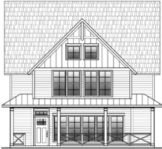
1 FRONT ELEVATION - BUILDING 1 3/16" = 1'-0"
